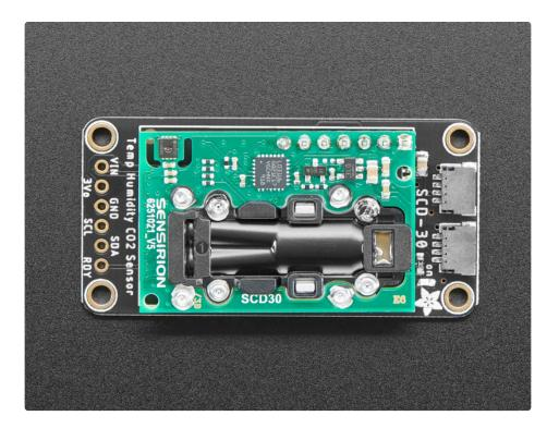
Data is read over I2C, so it works very nicely with just about any microcontroller or microcomputer. We've written both Arduino and Python/CircuitPython code so you can get started in a jiffy. Another nice element to this sensor is it comes with an <u>SHT31 temperature and humidity sensor already built</u> in (https://adafru.it/y7f). The sensor is used to compensate the NDIR CO2 sensor, but its also readable so you get full environmental data.
