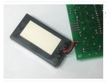
Time to wrap it up. Remove one side of paper from the sticky foam, place it in the center of the battery holder. Then remove the other side.
