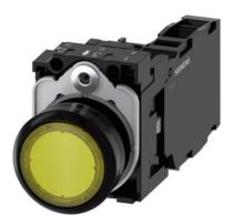
Illuminated pushbutton, 22 mm, round, plastic, yellow, pushbutton, flat, momentary contact type, with holder, 1 NO+1 NC, LED module with integrated LED 24 V AC/DC, screw terminal, with laser labeling, inscription or symbol Customer-specific selection with SIRIUS ACT configurator (CIN)
