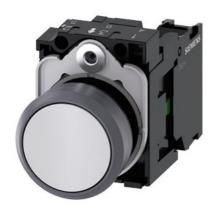
Pushbutton, 22 mm, round, plastic with metal front ring, white, pushbutton, flat, momentary contact type, with holder, 1 NO, screw terminal, with laser labeling, lower case
