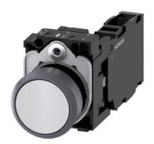
Pushbutton, 22 mm, round, plastic with metal front ring, white, pushbutton, flat, momentary contact type, with holder, 1 NO+1 NC, screw terminal, with laser labeling, symbol number according to, ISO 7000 or IEC 60417
