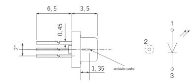
all dimensions in mm. Tolerance  $\pm 0,\,1$  except given ones \* at the bottom of the LED
