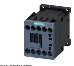
Power contactor, AC-3 12 A, 5.5 kW / 400 V 1 NO, 200 V AC, 50 Hz 200-220 V, 60 Hz, 3-pole Size S00, screw terminal
