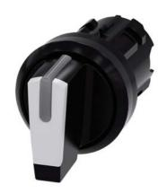
Selector switch, illuminable, 22 mm, round, plastic, white, selector switch, short, 3 switch positions I-O-II, latching, actuating angle  $2x45^{\circ}$ , 10:30h/12h/13:30h, with laser labeling, lower case
