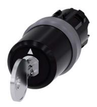
key-operated switch Siemens, 22 mm, round, plastic with metal front ring, lock number SSG10, with 2 keys, 3 switch positions I-O<II, left latching, momentary contact type on the right, actuating angle  $2x45^{\circ}$ , 10:30h/12h/13:30h, key removal O+I, with laser labeling, lower case
