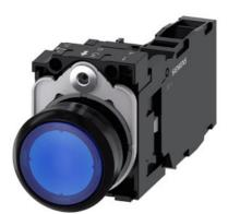
Illuminated pushbutton, 22 mm, round, plastic, blue, pushbutton, flat, momentary contact type, with holder, 1 NO+1 NC, LED module with integrated LED 24 V AC/DC, screw terminal, with laser labeling, upper case
