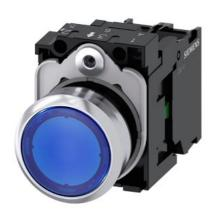
Illuminated pushbutton, 22 mm, round, metal, shiny, blue, pushbutton, flat, momentary contact type, with holder, 1NO, LED module with integrated LED 24 V AC/DC, screw terminal, with laser labeling, symbol number according to, ISO 7000 or IEC 60417
