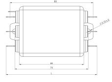
**General Information** Series FLLD3-AW Style **Chassis Mount** Description Compact, Three-Phase and Neutral Filters Three Phase, Compact Features Phase Three-phase RoHS Yes Qualifications UL 1283 **Terminal Type** Faston
