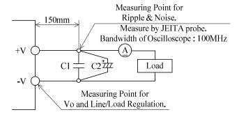
C1 : Film Cap.  $0.1\mu F$ C2 : Elect. Cap.  $100\mu F$  A263-01-02/A
