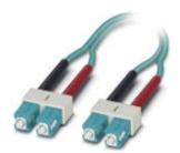
Assembled FO cable, zip cord cable, multi-mode fiberglass 50/125  $\mu$ m, OM3, plug: SC duplex/SC duplex, degree of protection: IP20, for installation in cable ducts or control cabinets, length: 1 m
