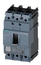
circuit breaker 3VA5 UL frame 125 breaking capacity class H 65kA @ 480 V 3-pole, line protection TM230, FTAM, In=20A overload protection Ir=20A fixed short-circuit protection Ii=7.5...15 x In UL489 SB (naval), 50 deg. cel. nut keeper kit on both sides
