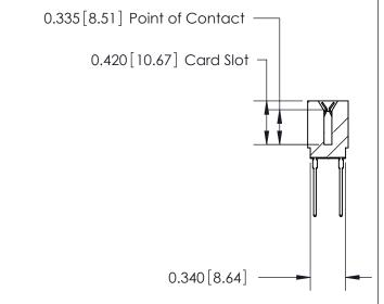
726 Series Ultra-Mate Card Edge Connector - Press Fit Part Number: 726-058-545-201
