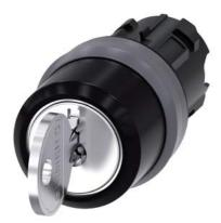
RONIS key-operated switch, 22 mm, round, plastic with metal front ring, lock number SB30, with 2 keys, 3 switch positions I-O-II, latching, actuating angle 2x45°, 10:30h/12h/13:30h, key removal O, possible special locks: SB31, 421, 455, with laser labeling, upper case and lower case, always upper case at beginning of line
