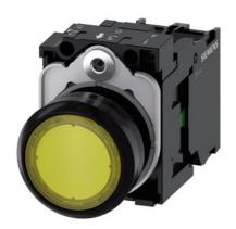
Illuminated pushbutton, 22 mm, round, plastic, yellow, pushbutton, flat, momentary contact type, with holder, 1NO, LED module with integrated LED 230 V AC, screw terminal, with laser labeling, symbol number according to, ISO 7000 or IEC 60417
