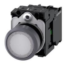
Illuminated pushbutton, 22 mm, round, plastic with metal front ring, white, pushbutton, flat, momentary contact type, with holder, 1NO, LED module with integrated LED 110 V AC, screw terminal, with laser labeling, upper case and lower case, always upper case at beginning of line
