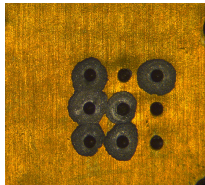
Figure 52: Result of solder paste wicking through thermal vias during reflow. Photograph of board 1, bottom side.
