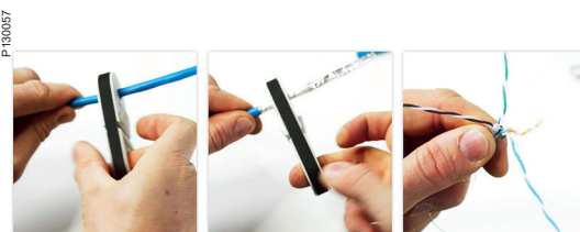
Use the cable stripper tool and cut the outer sheath. Cut the one single foil metallic crossfiller and remove it with a simple grip. Your CL-MX is ready to connect.
