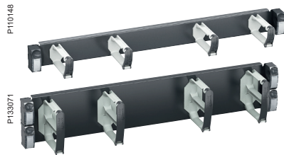
Guiding panels for patch cords The 1U panel manages 24 cords, and 2U panel 48 cords. Easily opened but still safe, since a clever device prevents cords from falling out. Also possible to pull out only one cord if needed.
