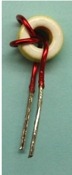
Figure 14 – Finished Part, Front View. Tin Leads to within ~1/8” of Toroid Body.
