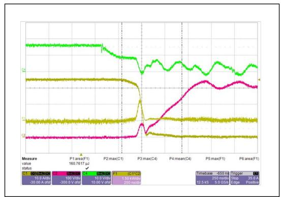
Figure 7: STGW40H60DLFB turn-off waveform, Power = 1 kW, C<sub>SNUBBER</sub> = 33 nF
