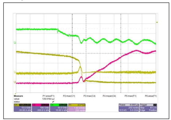
Figure 9: STGW40H60DLFB turn-off waveform, Power = 3 kW, C<sub>SNUBBER</sub> = 33 nF
