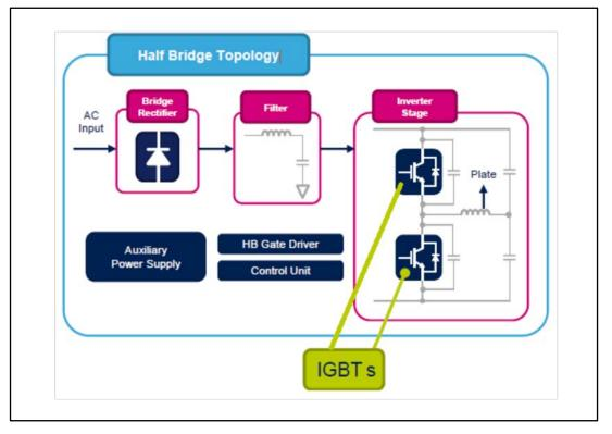
Figure 2: IGBTs in half bridge topology.
