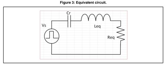
If the chosen switching frequency is above the resonant frequency, the series resonant circuit behaves as an inductive load and the load current lags the output voltage.
