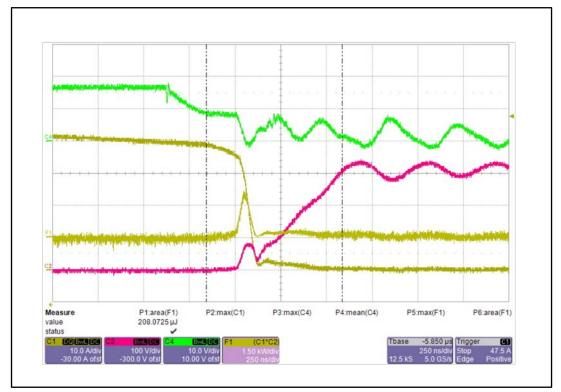
Figure 8: STGW40H60DLFB turn-off waveform, Power = 2 kW, C<sub>SNUBBER</sub> = 33 nF
