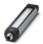
LED machine light, 24 V DC, emission angle 85 °/95 °, color temperature 5000 K, length 190 mm, diameter 40 mm, M12 connector, Light housing: Anodized aluminum, Pane: Single-pane safety glass (ESG, thermally toughened float glass), pivoting, resistant to coolants and lubricants, can be switched in series
