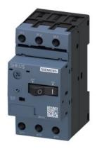
Circuit breaker size S00 for motor protection, CLASS 10 A-release 0.18...0.25 A N-release 3.3 A Screw terminal Standard switching capacity
