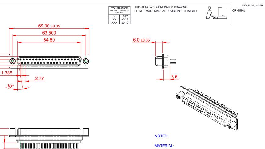
HOUSING: THERMOPLASTIC POLYESTER, UL94V-0 SHELL: STEEL, TIN PLATED CONTACT: COPPER ALLOY, 30µ GOLD PLATED OPERATING TEMPERATURE: -55°C to +85°C (1)
