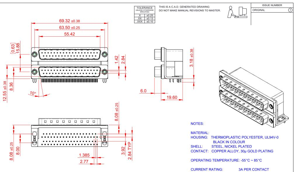
CONTACT RESISTANCE: 25mΩ MAX. INSULATOR RESISTANCE: 5000MΩ min. DIELECTRIC WITHSTANDING VOLTAGE: 1000V AC rms
