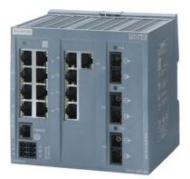
SCALANCE XB213-3LD managed layer 2 IE switch 13x 10/100 Mbit/s RJ45 ports, 3x SM FO SC-port 1x console port, diagnostics LED, redundant power supply, IEC 62443-4-2 certified; temperature range 0 °C to +60 °C; DIN-rail mounting; default EtherNet/IP.
