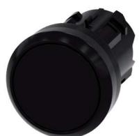
Pushbutton, 22 mm, round, plastic, black, pushbutton, flat, latching, Pushto-release mechanism, with laser labeling, upper case
