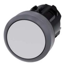
Pushbutton, 22 mm, round, plastic with metal front ring, white, pushbutton, flat, latching, Push-to-release mechanism, with laser labeling, symbol number according to, ISO 7000 or IEC 60417
