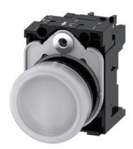
Indicator lights, 22 mm, round, plastic, white, lens, smooth, with holder, LED module, with integrated LED 230 V AC, screw terminal, with laser labeling, lower case
