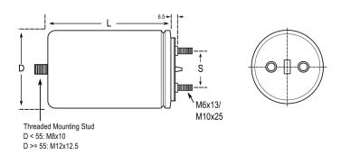
General Information Series C44A Dielectric Metallized Polypropylene Style Can RoHS With Exemptions **REACH** SVHC (Pb - CAS 7439-92-1) cc1c1ec4-db9e-4815-b26b-e8a34ddfb776 SCIP Number Lead Threaded Studs M6 AEC-Q200 No Component Weight 583.3 g Thermal Resistance = 4 C/W. Miscellaneous
