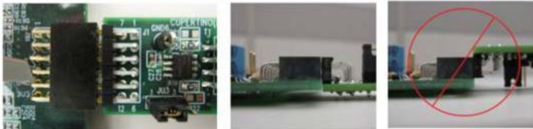
Figure 2. Pmod™ Connector Alignment
