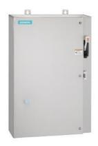
Non-reversing motor starter Size 0 Three phase full voltage Solid-state overload relay OLRelay amp range 3-12A Combination type 30Amp nonfusible disconnect Encl NEMA type 4X 316 S-steel Water/dust tight noncorrosive Extra-wide enclosure
