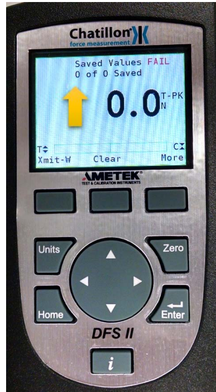
Figure 5 Gauge Indicates 0 of 0 Saved Values. If additional values are indicated repeat step 3 and step 4. Gauge will now be able to be changed to different modes.
