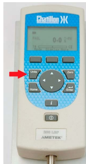
To change units, select Units . ( Newtons are recommended by HellermannTyton Engineering Department ).
