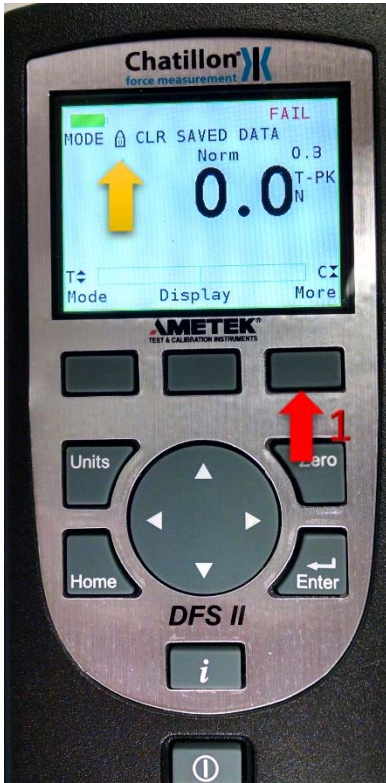
Figure 1 Gauge indicates Mode-Lock and notes to Clear Saved Data. Press the More Button to switch screens.
