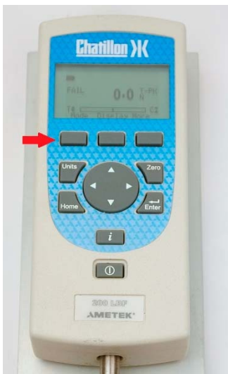
Select Mode until T-PK is displayed. This sets the gage to "Tension Peak Mode".
