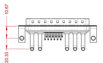
OPERATING TEMPERATURE: $-55^{\circ}C \sim 125^{\circ}C$ POWER/CO-AX CONTACT RATING:30A (CURRENT)(IF PRESENT)SIGNAL CONTACT CURRENT RATING:5A PER CONTACTSIGNAL CONTACT RESISTANCE: $10m\Omega$  MAX.INSULATOR RESISTANCE: $5000M\Omega$  min.DIELECTRIC $5000M\Omega$  min.
