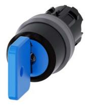
Key-operated switch O.M.R, 22 mm, round, plastic with metal front ring, lock number 73038, blue, with 2 keys, 3 switch positions I-O-II, latching, actuating angle 2x45°, 10:30h/12h/13:30h, Key removal I+O+II, Z=50-unit packaging
