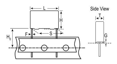
General Information Series F872 Dielectric Metallized Polypropylene Style Radial Features MKP EMI Safety RoHS Yes Lead Wire Leads Safety Class X1 Qualifications ENEC, UL, cUL, CQC AEC-Q200 No THB Performance No Component Weight 9.669 g Miscellaneous ClimCat: 40/110/56/B Shelf Life 104 Weeks
