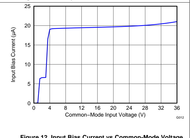
Figure 12. Input Bias Current vs Common-Mode Voltage
