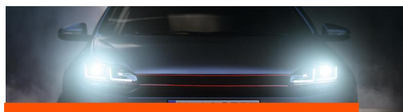
The LEDs in the standard low beam / high beam application guide enable a high LED penetration rate down to A-Segment. Due to a high electrical efficiency of the light sources, low thermal management efforts and the possibility to use low cost PCBs, a cost optimized system can be designed. By reducing the driving current while still keeping the required brightness even "Heatsinkless" headlamps become possible.
