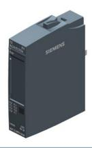
SIMATIC ET 200SP, Digital output module, DQ 8x 24V DC/0,5A Basic, Source output (PNP,P-switching) Packing unit: 10 pieces, fits to BU-type A0, Colour Code CC02, aubstitute value output, module diagnostics for: supply voltage
