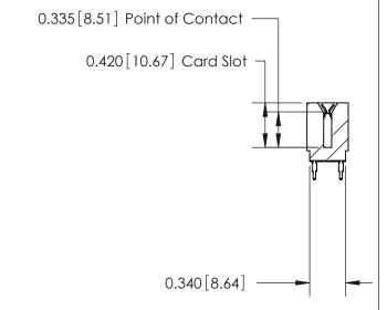
726 Series Ultra-Mate Card Edge Connector - Press Fit Part Number: 726-042-525-201 **EDAC INC** THESE DRAWINGS AND SPECIFICATIONS ARE THE PROPERTY OF EDAC INC.,AND TORONTO, ONTARIO SHALL NOT BE REPRODUCED, OR COPIED CANADA OR USED AS THE BASIS FOR THE
