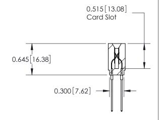
737 Series Ultra-Mate Card Edge Connector - Press Fit ACAD REFERENCE NO.
