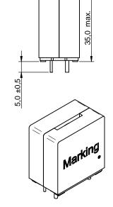
Pin 2 and 3 are only for mechanical stability.
