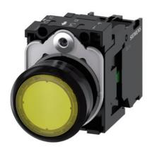
Illuminated pushbutton, 22 mm, round, plastic, yellow, pushbutton, flat, momentary contact type, with holder, 1NO, LED module with integrated LED 230 V AC, screw terminal, with laser labeling, inscription or symbol Customer-specific selection with SIRIUS ACT configurator (CIN)
