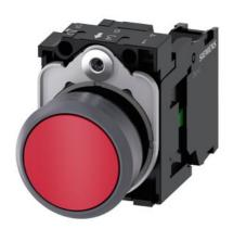
Pushbutton, 22 mm, round, plastic with metal front ring, red, pushbutton, flat, momentary contact type, with holder, 1 NO, screw terminal, with laser labeling, upper case and lower case, always upper case at beginning of line
