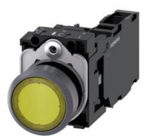
Illuminated pushbutton, 22 mm, round, plastic with metal front ring, yellow, pushbutton, flat, momentary contact type, with holder, 1 NO+1 NC, LED module with integrated LED 110 V AC, screw terminal, with laser labeling, upper case and lower case, Always upper case at the beginning of the word
