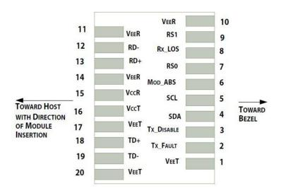
Pin-out of connector Block on Host board
