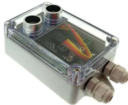
Pic. 15. WiFi Ultrasound sensor : waste collection project
