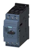
Circuit breaker size S2 for motor protection, Class 20 A-release 42...52 A N-release 741 A screw terminal Standard switching capacity
